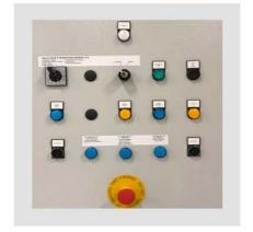
**OPERATING PANEL**Modern user-friendly operating panel with status indicators and commands for bale ejection and manual operation.
